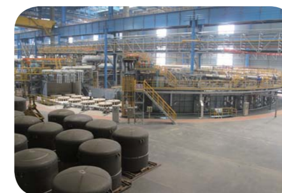
取向硅钢高温环形热处理炉 High temperature annular heat treatment furnace for oriented silicon steel
