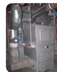
单蓄热式烧嘴 Single regenerative burners
