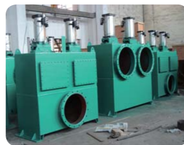
三通换向阀 3-way reversing valve
