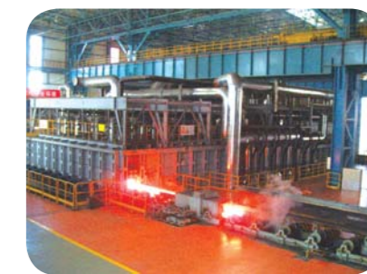
棒线材步进梁式加热炉 Walking beam reheating furnace for steel bars and wire rods
