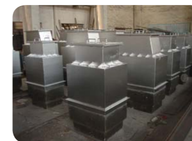
双蓄热式烧嘴 Double regenerative burners
