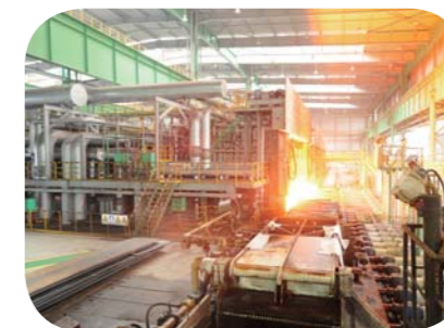
大型热轧板坯步进梁式加热炉 Walking beam reheating furnace for large hot-rolled slabs
